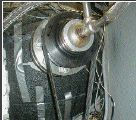
Belt-driven mixer using Co-Axial Type Coupling
